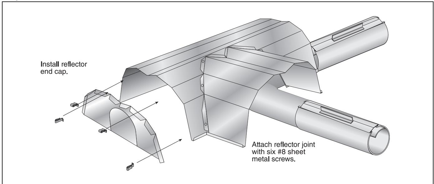
**FIGURE 30: Reflector Joint Detail**
