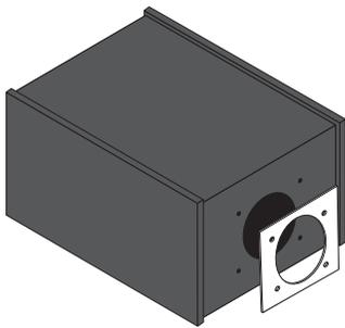
**Burner with Tube Gasket**
