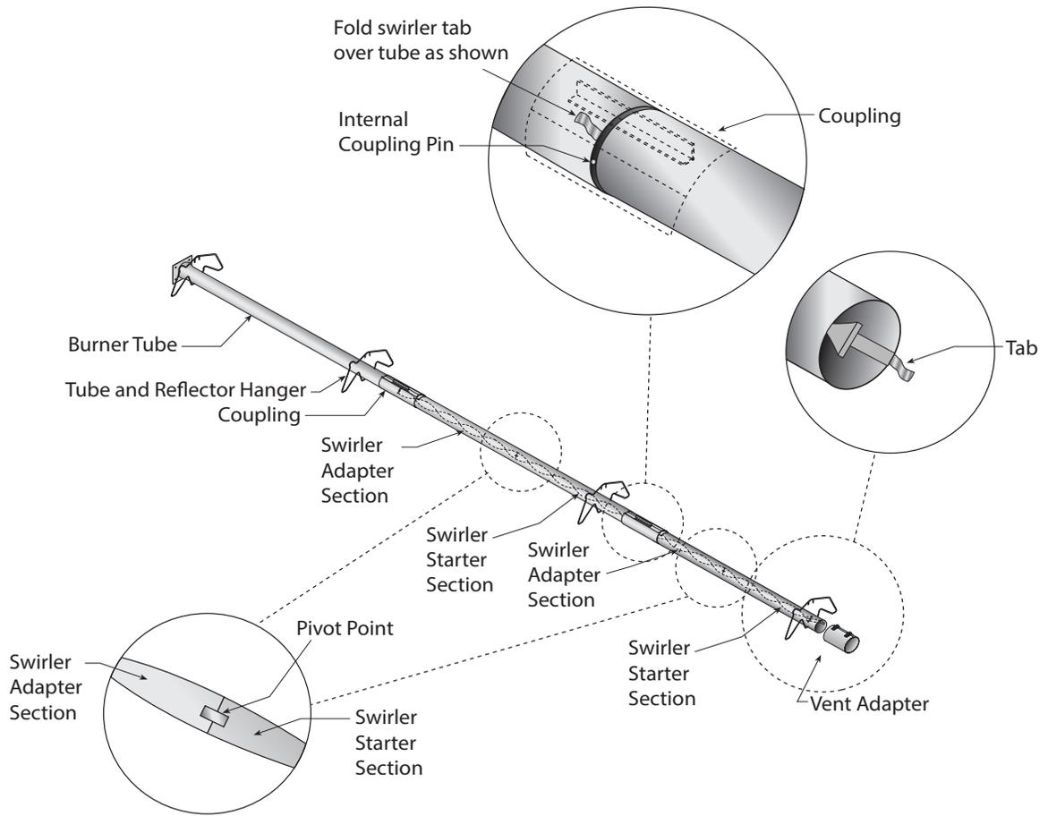
**FIGURE 21: Swirler Installation Model: CTH2V-125, 30' U-Tube; Swirler Package - 20' (6 m) (p/n 03051511K)**
