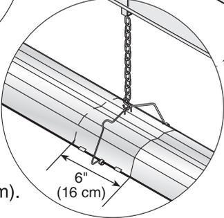
2. The overlap at the first and second reflector is a **slip overlap**. Thereafter, every third reflector joint is a slip overlap. A slip overlap is achieved by either:
