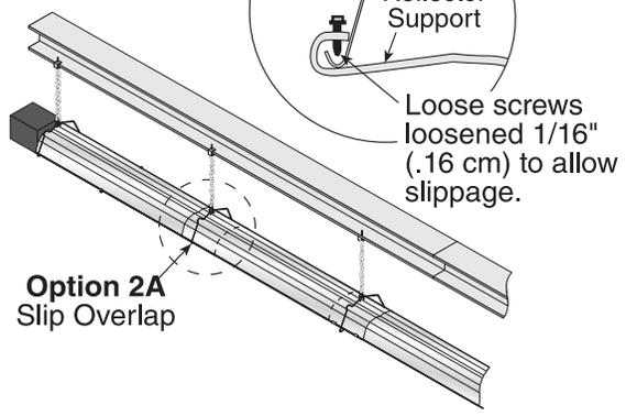
3. The remaining reflector overlaps require a **non-slip overlap** connection. To affix the reflectors together in a non-slip overlap either:
