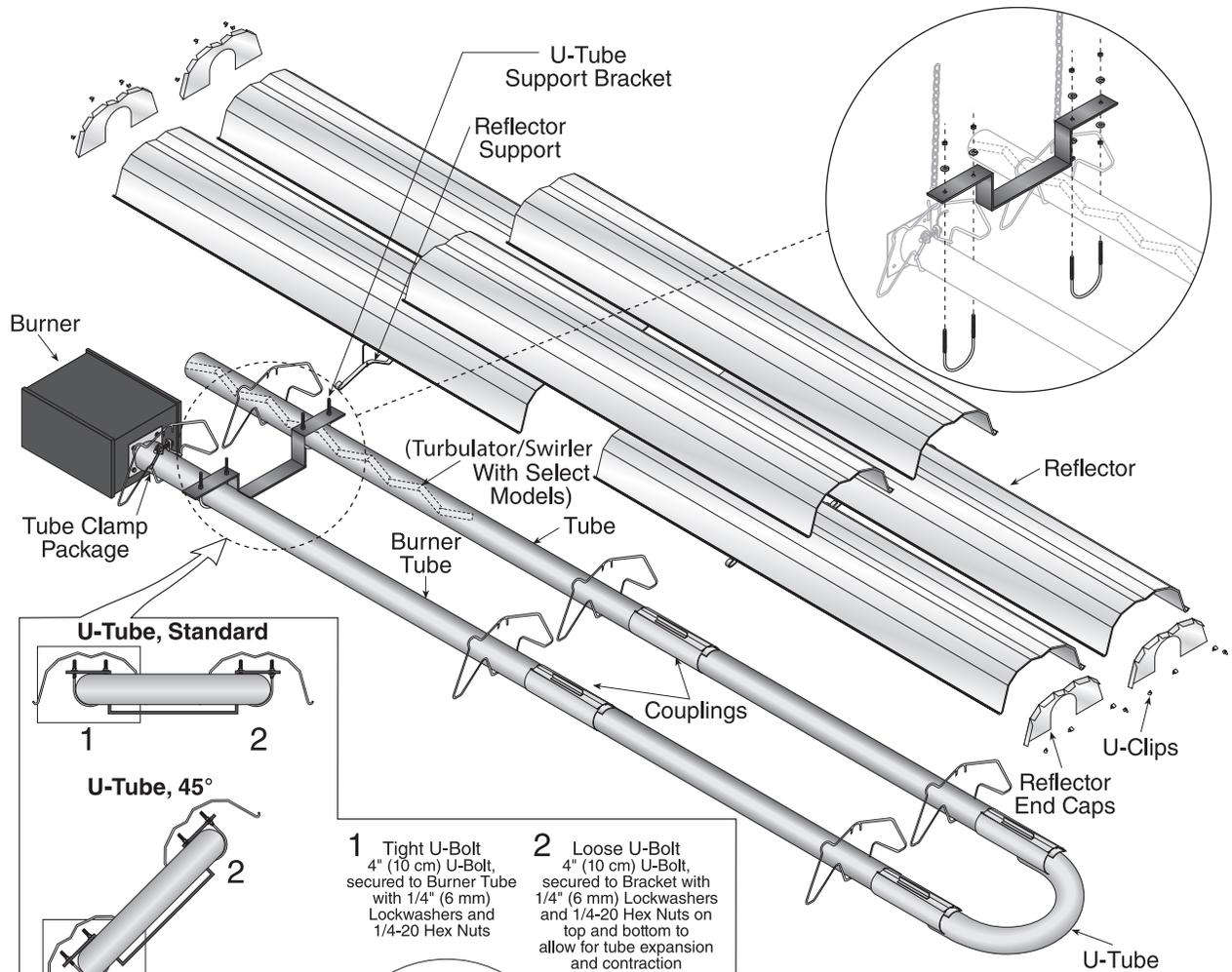
Mounting hardware shown is for indoor installation only. See Page 17, Figure 16 for outdoor suspension details.
