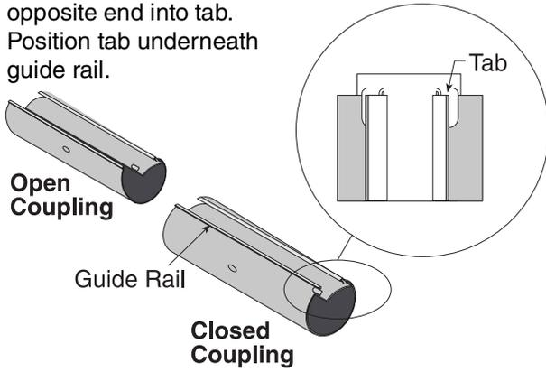
**B** Insert wide end of slide bar/coupling lock into guide rail on opposite end of tabs. Slide the slide bar/coupling lock up the guide rail until snug (approximately 3" (8 cm) to 4" (10 cm)).
