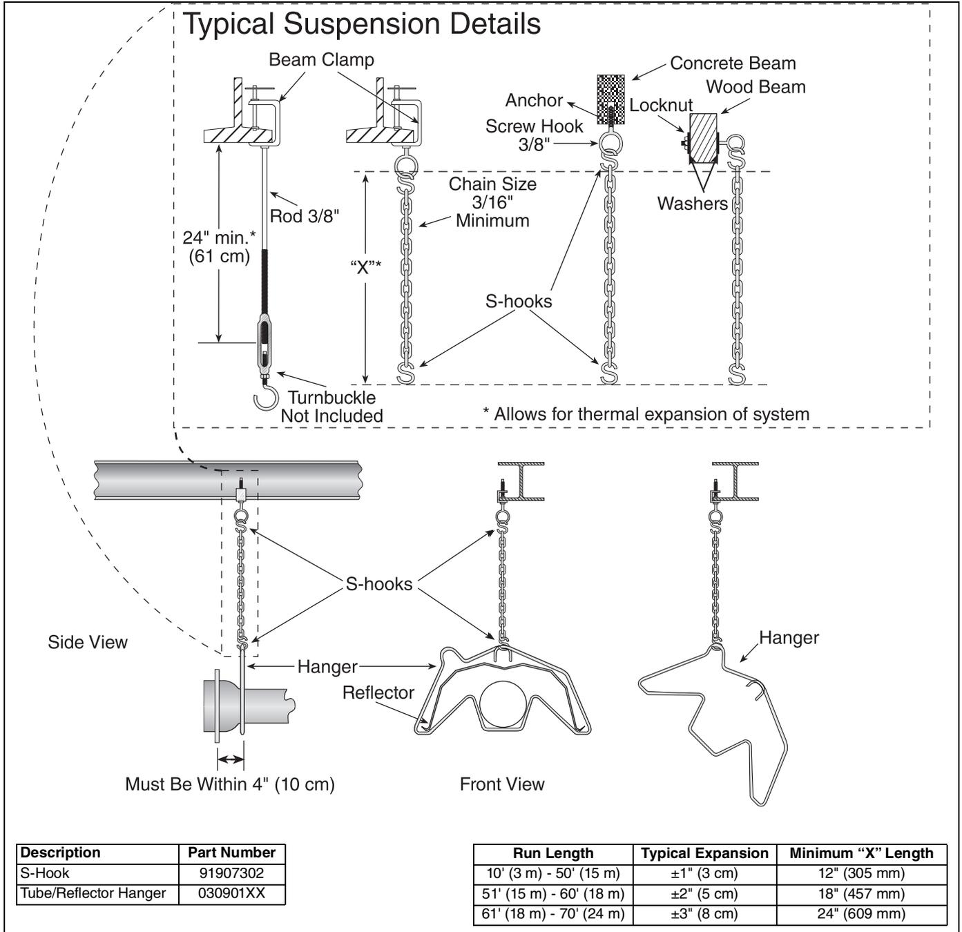
FIGURE 17: Linear Heater Assembly Overview
