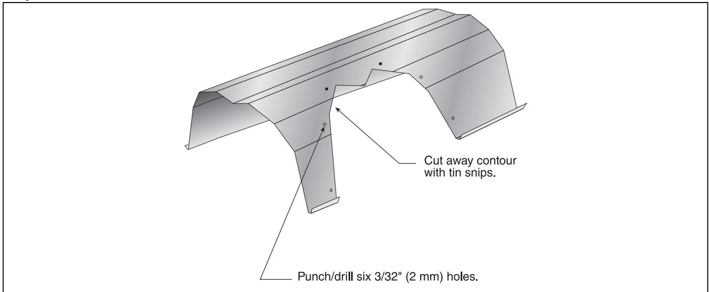
**Step 7.2.5 Reflector Joint Detail**
